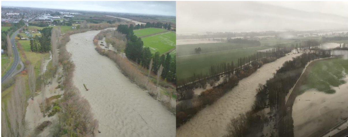
Figure 1: Aerial imagery of the Hakatere / Ashburton North Branch during 2021 floods. The left image is looking downstream, the right image is looking upstream. These images show fast, high energy water in the centre of the river, trees in the berm slowing the water to protect the stopbanks.
