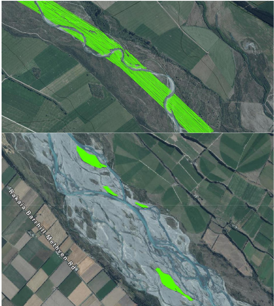
Figure 3. Screenshots from Environment Canterbury's GIS system showing the GPS tracks of an aerial spray operation on the North Branch Rakaia River (top) and the Rakaia River mainstem (bottom). The lines represent the flight path taken by the helicopter and records only when spray is discharging from the boom. Source: ECan Maps, Data supplied by helicopter operators.
