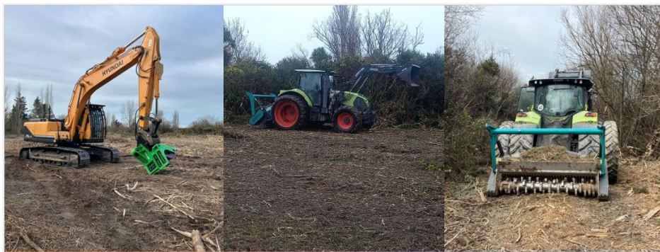
Figure 12, the machinery used at Stoddard’s island: Tree shear (left), Tractor with attached mulching deck (centre and right).
