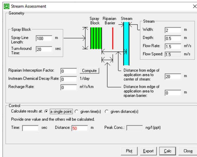
**Figure 2.** AGDISP stream assessment module, highlighting geometry of spray block and stream.
