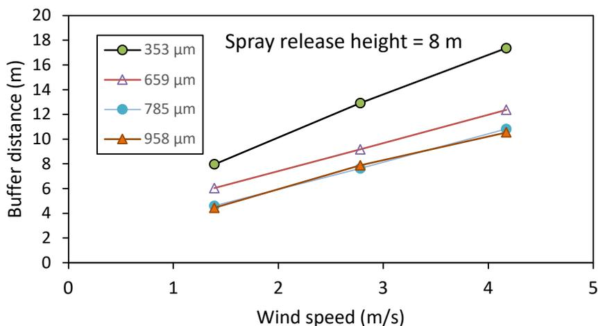
**Figure 8.** Effect of wind speed and droplet size on buffer distance for an 8 m release height.
