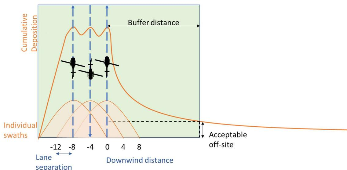
**Figure 1.** Overlapped swaths from 3 flight lines are summed to give total deposition both within and downwind of the spray block. Estimation of a suitable buffer distance depends on defining an acceptable threshold value of off-site deposition.
