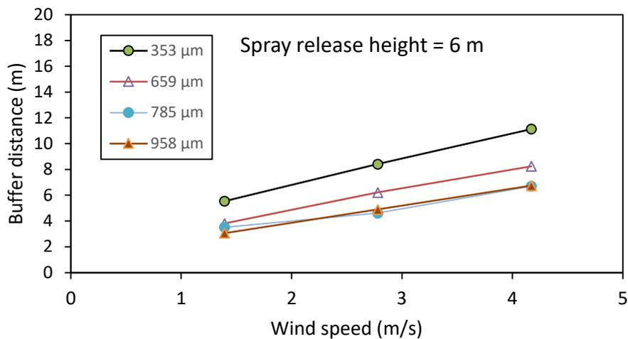
**Figure 7.** Effect of wind speed and droplet size on buffer distance for a 6 m release height.
