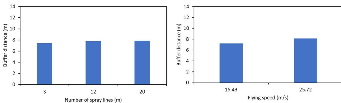
**Figure 6.** Buffer distance for each number of spray lines and flying speed.
