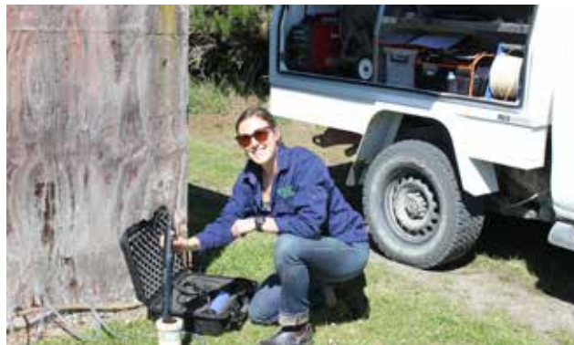
A staff member measures field parameters (pH, temperature and electrical conductivity) before collecting a groundwater sample
