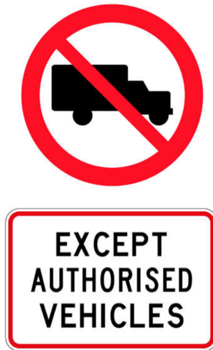
Figure 1: R5-3 No Heavy Vehicle Signage
