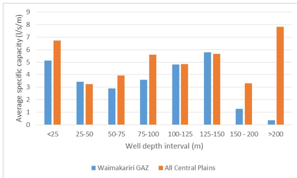
**Figure 1. Specific capacity data for the Waimakariri GAZ versus data used by ECan for the wider areas (Figure 6-3 of ECan, 2019b)**
