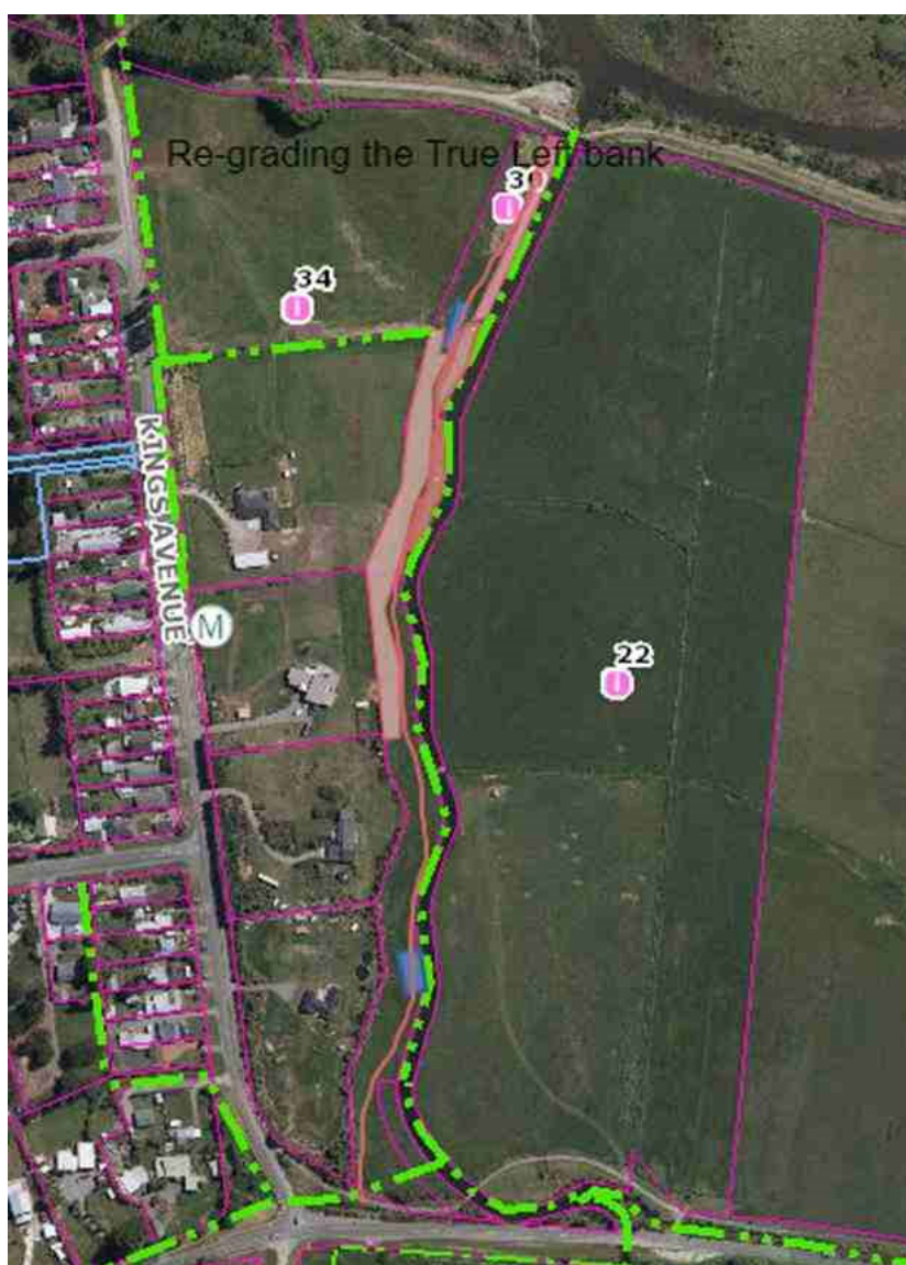
Figure 3: Indicates the 2020-21 planting (red areas), as well as the two installed culverts (blue rectangles) and path (orange line) connecting Ashley Rakahuri River stopbank walkway to a trail along Waikuku Beach Road, installed in 2019-20. Re-grading of the true left bank is planned as part of inanga spawning area improvements.
