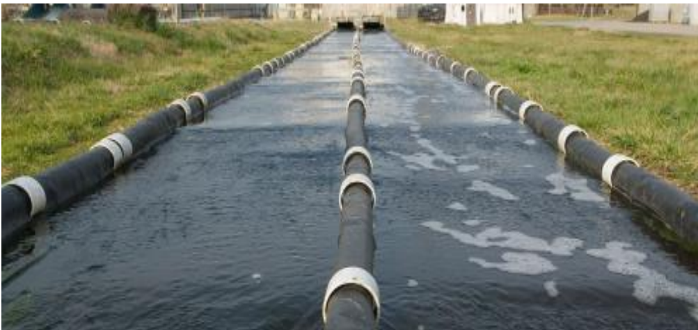
Figure 15: Example of a two-channel trial-based algal turf scrubber for nutrient removal. Photo source University of Maryland.
