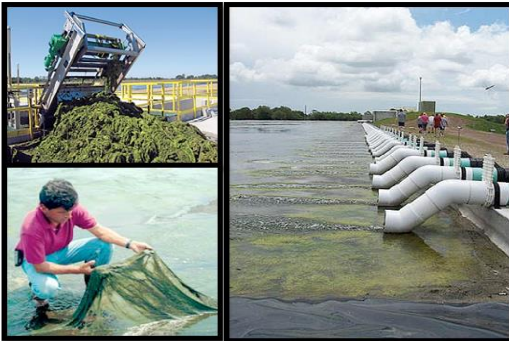
Figure 7: Algal turf scrubber (right) used to treat polluted water in Chesapeake Bay, USA and harvester removing periphyton from the flow-way (top left). Photo source Sandia National Laboratories.
