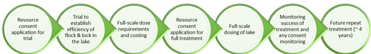
Figure 18: Implementation pathway for active sediment capping (flock & lock) in Pegasus Lake.
