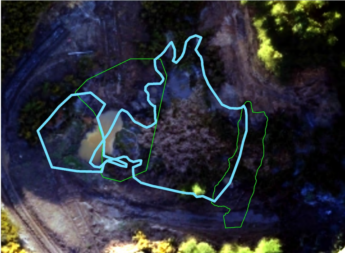
Figure 2: The approximate locations of the sediment retention ponds (blue outline) and associated bunds (green outline). The smaller sediment retention pond, which had already been constructed at the time of the site investigation, is on the left. The larger pond, which is the subject of this assessment, is on the right (spatial data sourced from Bathurst).
