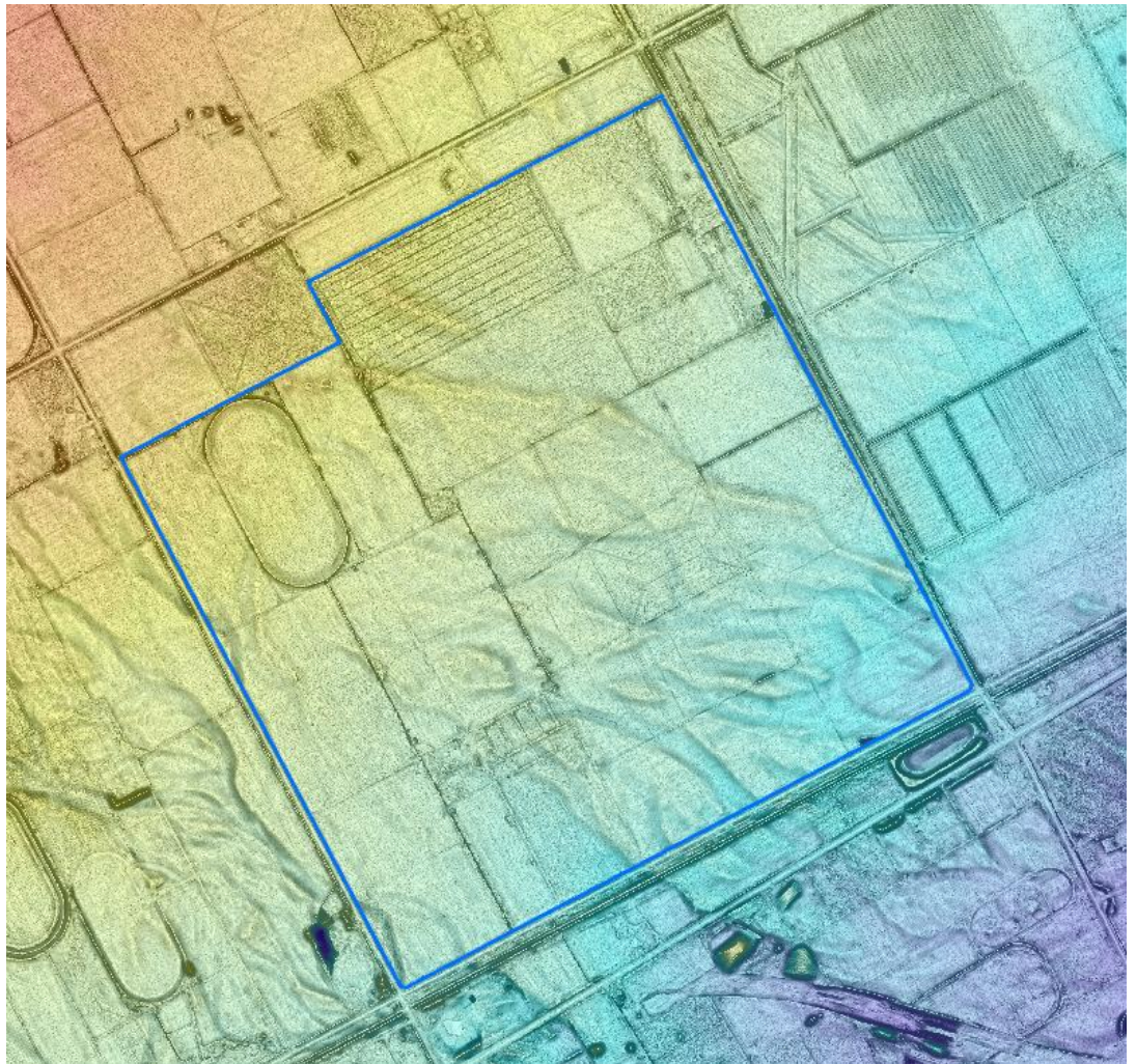
Figure 2 – Terrain analysis of LiDAR showing the old river channels through the site
