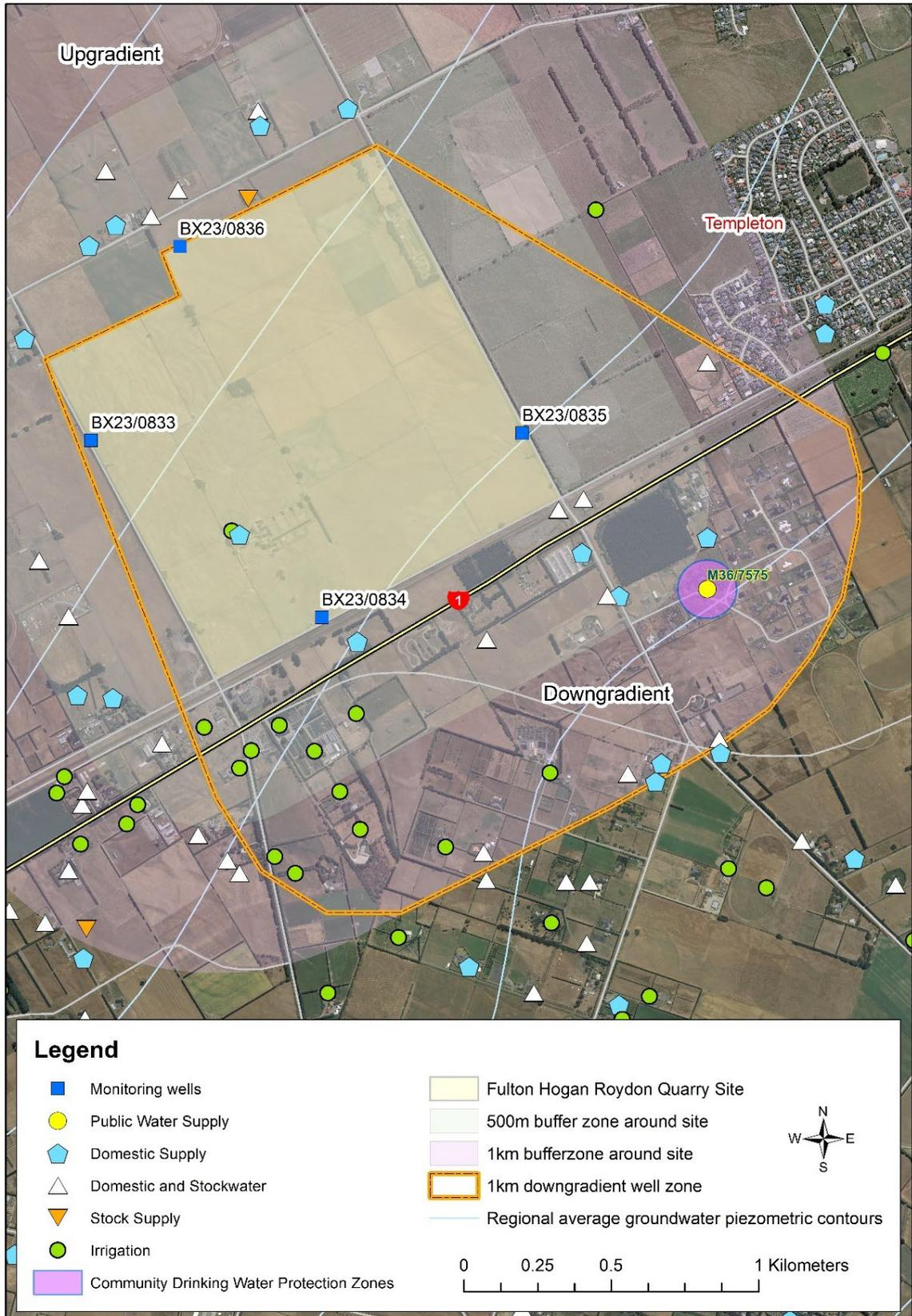
**Attachment 2:** Location of wells and their registered water uses near the proposed Roydon Quarry (sourced from Environment Canterbury’s wells database).
