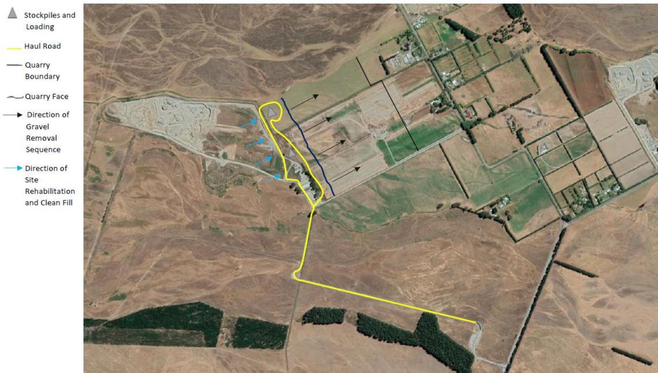
**Note:** The Haul Road will drop into the 10 metre Quarry Pit. The exact route of the Haul Road will change as the Quarry progresses, however, it will always pass the Quarry Office and Weigh Bridge in both directions.
