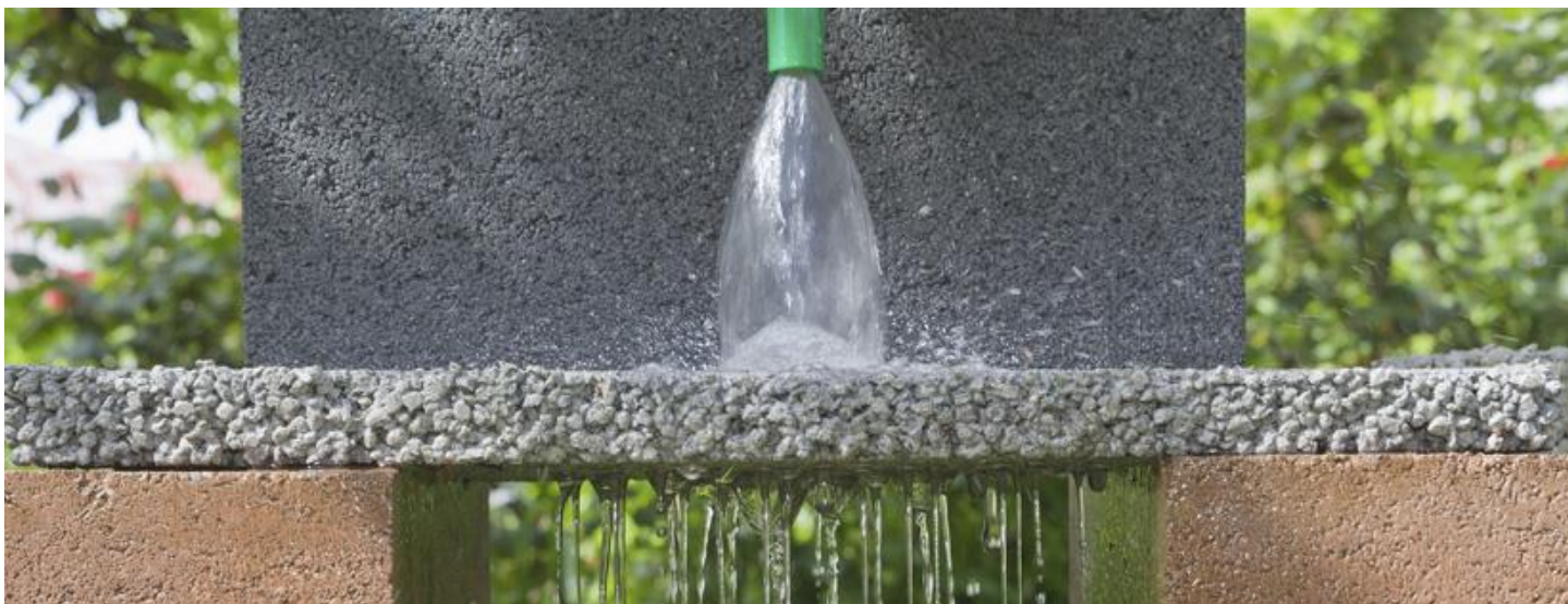
Figure 2: Permeable pavement demonstration (Harrison, 2011)
