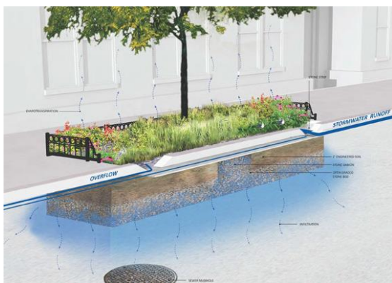
Figure 3: Rain garden cross section
