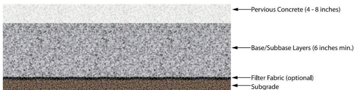
Figure 2: Pervious concrete pavement cross section. Recommended subbase layer of SUDS installation depth to be 1 meter containing 40% void volume aggregate (adapted from EPA, 2010)
