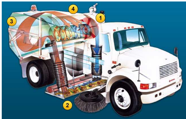
Figure 2: Schematic showing operating principles of regenerative air sweeper (from Tymco website www.tymco.com ).
