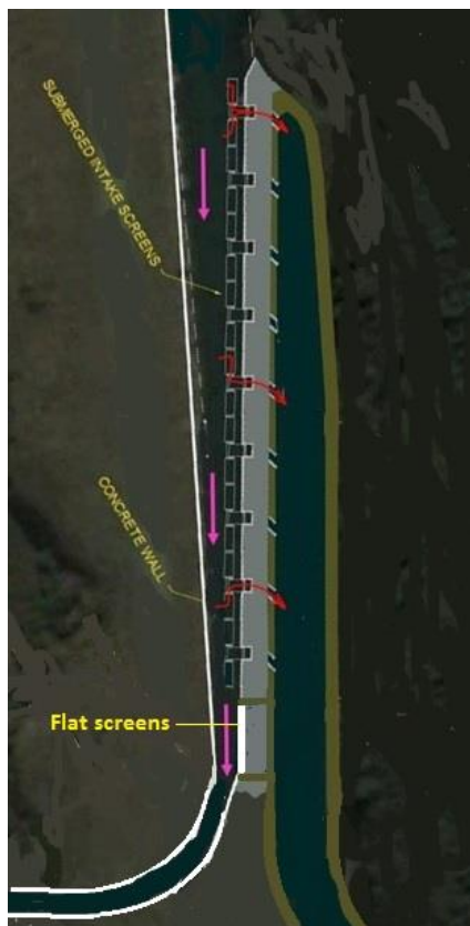
Figure 3: Schematic layout of fish screen and bypass channel
