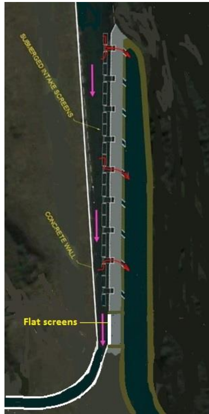
Figure 3: Schematic layout of fish screen and bypass channel (blue box shown in Figure 4)
