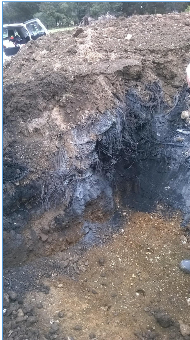
Figure 1: Excavation into pile showing capping material, burned tyres and underlying soil.
