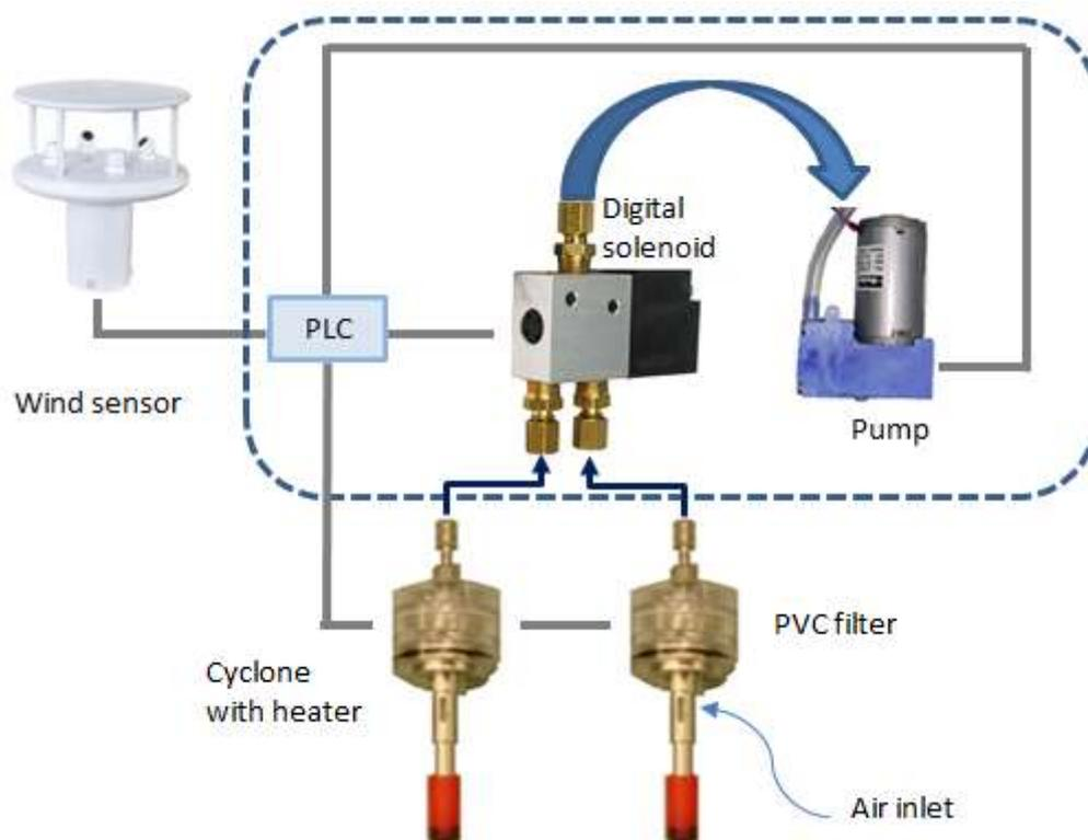
Figure I-2: Primary features of the wind directional RCS monitoring system
