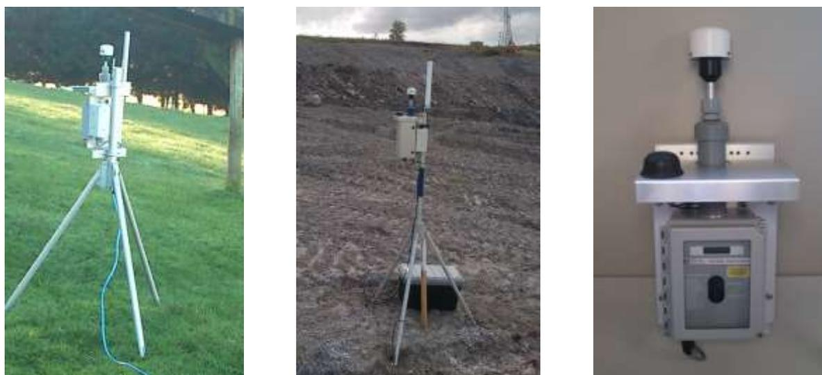
**Figure I-3: Typical nephelometer installations. The unit on the left is mains powered, while the unit in the centre is battery powered. The unit on the right provides a close up.**
