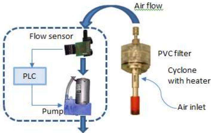
Figure I-1: Primary features of the RCS monitoring system
