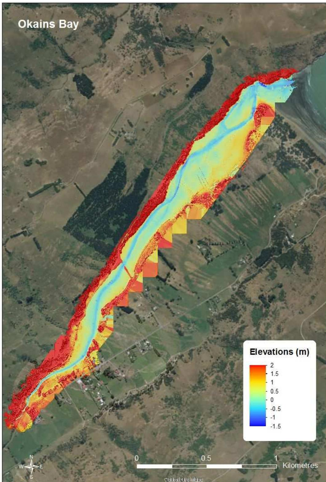
**Figure 3-2:** Elevation map of Okains Bay Estuary obtained by combining measurements from using echo-sound data for submerged parts of the estuary, and laser scan data for the intertidal areas. Cooler colours indicate lower elevation.
