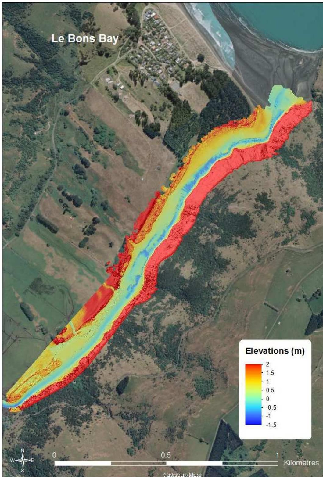
**Figure 3-1:** Elevation map of Le Bons Bay Estuary obtained by combining measurements from a kayak-mounted echo sounder, photogrammetry for the upper part of the estuary and laser scan data for the lower part of the estuary. Cooler colours indicate lower elevation.
