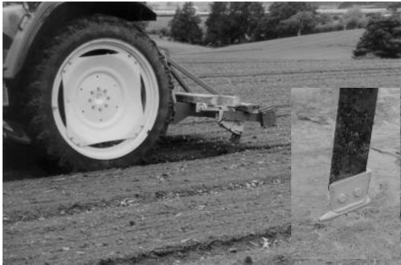
Photo 4. Wheel tracking ripping in action (above) and the small torpedo foot (insert).
