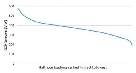
Orion network load duration curve for FY2015
