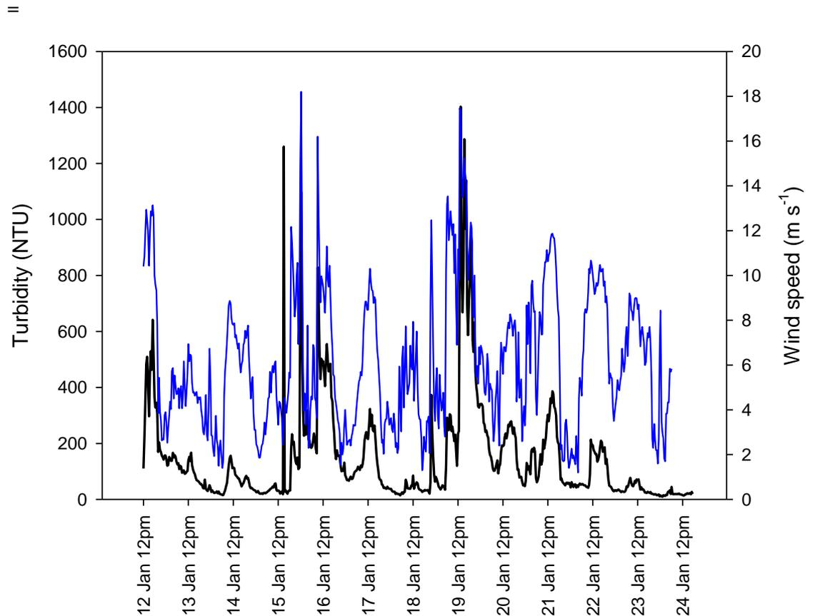
**Figure 3: Turbidity (black line) and wind speed (blue line) in Wainono Lagoon. Measurements taken every 30 minutes during a 12 day period in January 2011.**
