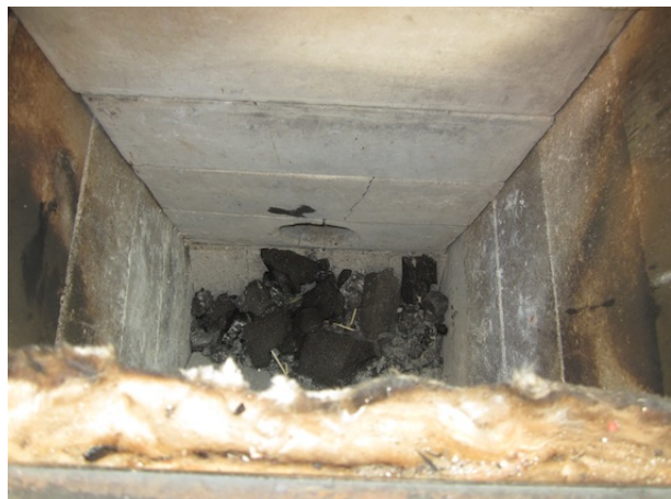
View into the fuel bin with small amount of charcoal sitting above a 10x340 mm slotted grate. Primary-secondary fuel gas port, centre just above the charcoal.
