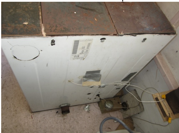
RH Side face showing thermocouple leads penetrating case and the primary air inlet at the base
