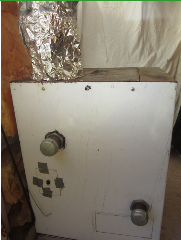
LH Side wall showing secondary air entry (lower port) and just installed flue gas extraction port for recirculation and oxygen dilution of (secondary) MILD combustion air. Insulated flue immediately above, issuing from the combustion chamber cover plate.
