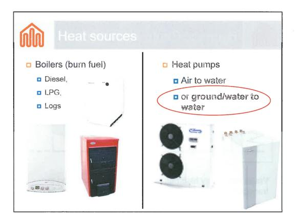
Heat sources include boilers that burn fuel, gas and diesel are commonly used in Christchurch even though they are not as cheap as heat pumps to run. Log boilers are difficult to install due to emissions regulations. Air to water and ground source heat pumps are growing in popularity every year.
