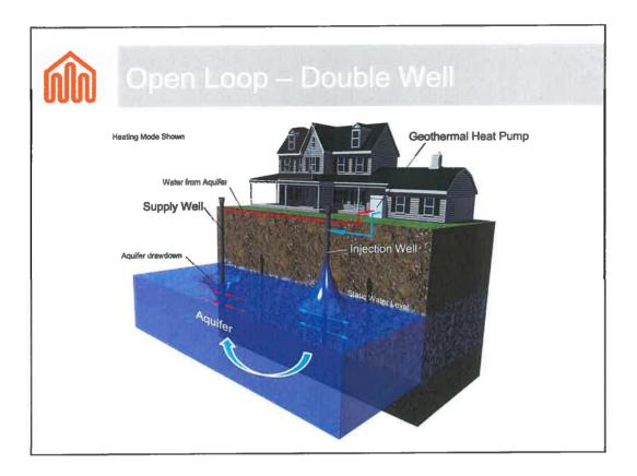
A potential problem is that if the bores are too close together the ejected water can circulate back to the extract well and reduce the efficiency of the heat pump.
