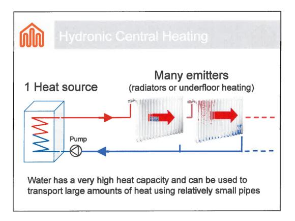
Hydronic central heating uses water to transfer heat from one central heat source to heaters usually in every room of the building. As water has a very high heat capacity it is possible to move large amounts of heat through relatively small pipes. It also means heat can be directed to where it is needed using automated valves and pumps.
