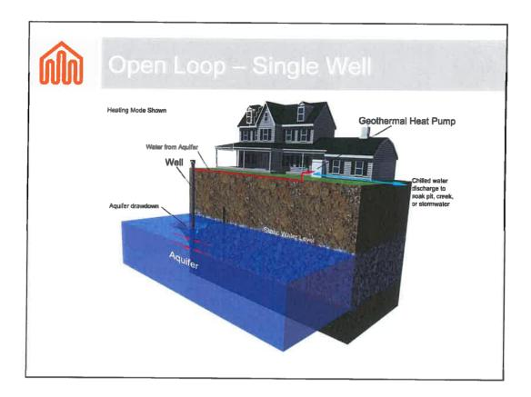
Some groundwater installations take the ground water from an aquifer and dump it into a drain or soak pit.
