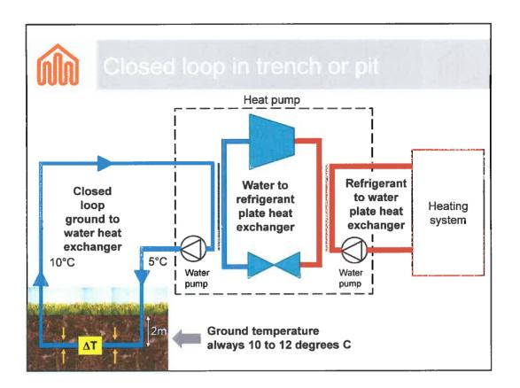
Pipe loops buried in the ground at a depth of 2m is the most common form of ground source heat pumps.
