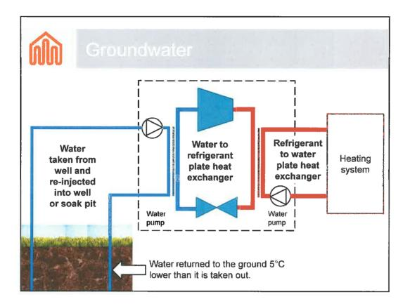
Using ground water is more cost effective as long pipe loops are eliminated and the groundwater is at a constant temperature of 10°C to 12°C.
