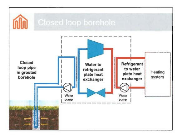
A variant of buried pipes it to put them in vertical bore holes which uses less land area but is expensive as the bores are 100m deep.
