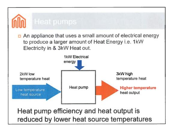
A heat pumps extracts large amounts of low temperature heat from the environment and concentrates it into a smaller amount of high temperature heat. Underground it is warmer in the winter than above ground where the air can be freezing, reducing efficiency and requiring defrost with reduces heat output of air source heat pumps.
