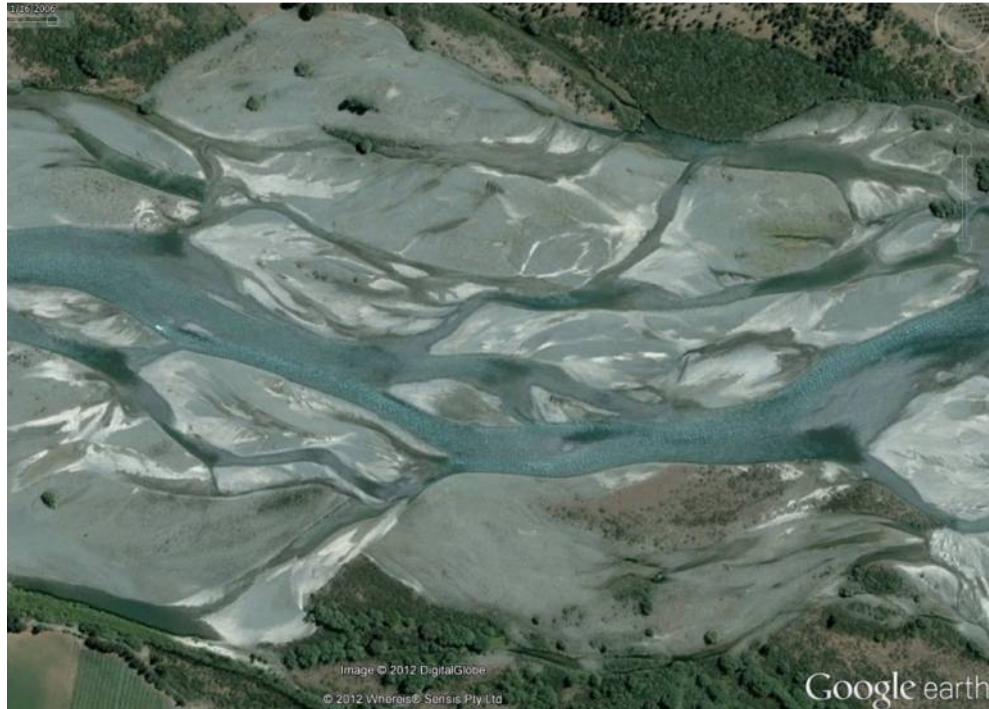
Figure 2. Example of Hurunui River braiding pattern, 12 km upstream of SH7, at a flow of 66 \text{ m}^3/\text{s} (recorded at Mandamus) on 16 January 2006.
