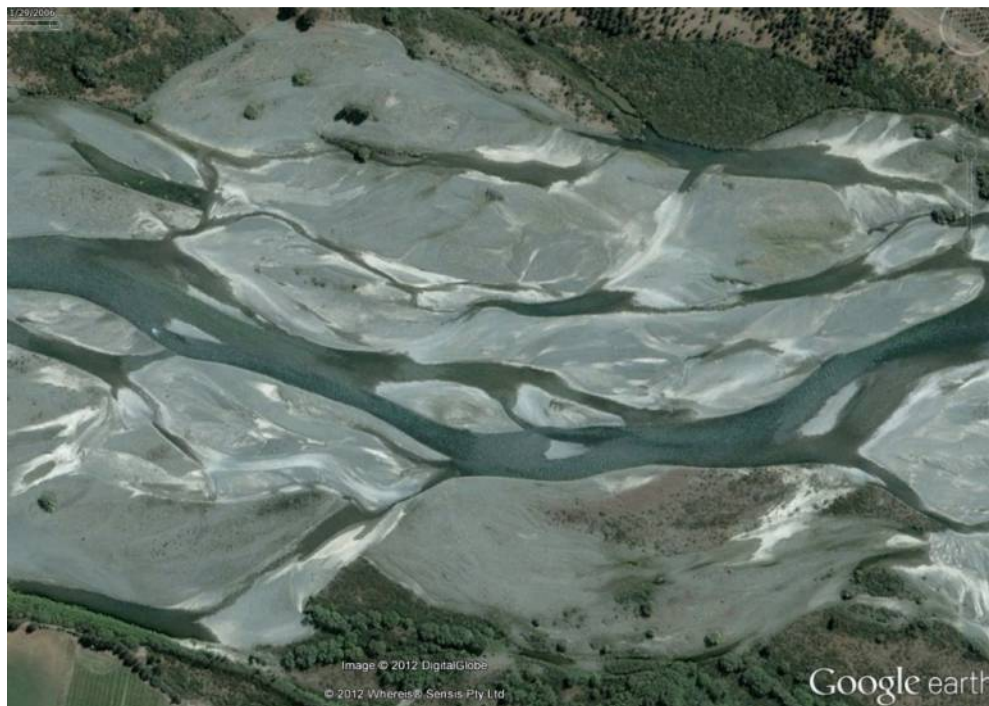
Figure 3. Example of Hurunui River braiding pattern, 12 km upstream of SH7, at a flow of 26 \text{ m}^3/\text{s} (recorded at Mandamus) on 29 January 2006.
