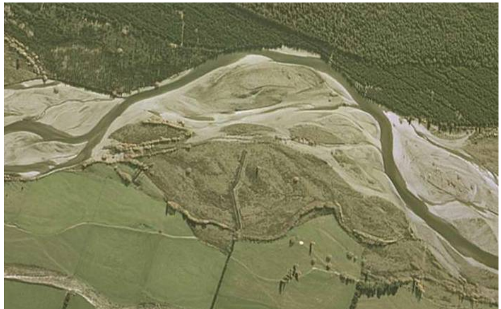
Figure 2: Aerial photograph of a non-braided sub-reach at between km 5 and km 7 in Amuri Reach. Image date 2/11/2004, flow 61 \text{ m}^3/\text{s} .
